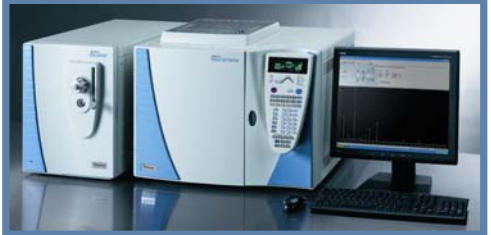
FIGURE 1. The Polaris Q ion trap, shown with TRACE GC Ultra. The instrument was modified to incorporate a liquid CI controller at the entrance to the transfer line. This allowed methanol vapor to enter the source and create the CI plasma.
