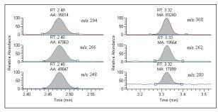
Figure 2: Quant and Qual ions for amphetamine (left) and methamphetamine (right) at 25 ng/mL level, showing good chromatography and signal intensity at the limit of detection for this method.
