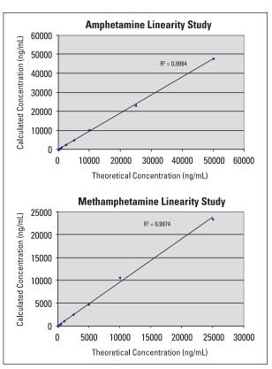
Figure 1: Linearity study results for amphetamine (top) and methamphetamine (bottom), comparing average concentrations for replicates at 10 different levels to the expected amounts at each level. The regression analysis for this study gave a correlation coefficient of 0.9994 across 11 levels for amphetamine and 0.9974 across 10 levels for methamphetamine.
